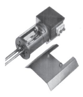
Cooled slit-jaw provided for up to 6 kW beam power; ceramic insulation of cooling pipes; stainless steel shield as protection against sputtering; used for slit current measurement.
