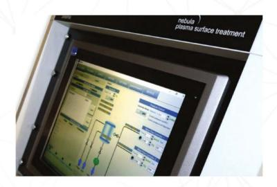
They are suited to both regular industrial usage and also for development of new processes and surface chemistry. NEBULA plasma treatment systems have a large HMI interface and are controlled via an industrial PLC system. They allow user level access ranging from simple operator, able to execute programs only, to full administrator, able to create users, edit, and test new recipes. Due to their flexibility and robustness, they are chosen where reliability and flexibility are paramount.
