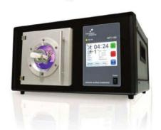
The TEM plasma cleaner is an application specific solution for low-pressure plasma cleaning and preparation of electron microscopy samples, including:
