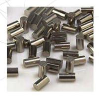
Princeton Scientific Corp. provides a wide variety of evaporation materials for the vacuum deposition industry. Our materials are available in various purities ranging from 99.9% to 99.99999%. Evaporation material can be made to order in the following forms:
