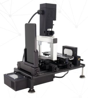
Smart measurement instrument with an automatic dropper for surface energy research.
