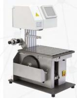
The diamond wire saw DWS.250E (endless) is a one-way table saw in vertical design.
